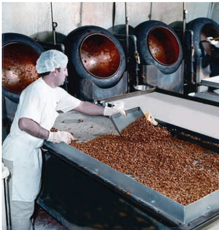
As part of Warrell’s hot panning operation, freshly produced butter-toasted caramelized peanuts are cooled before packaging. This is in the 215,000-sq.-ft. main plant in Camp Hill, Pa.
