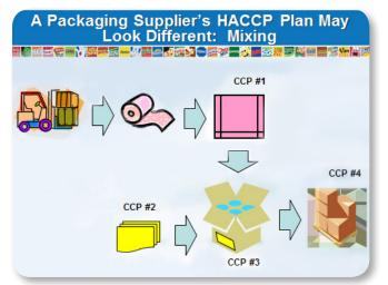
**Fig. 1:** A 'single' hazard such as mixing labels can have many CCPs, or Critical Control Points, as seen in this illustration, where mixing can occur on pouches (CCP 1), in cartons (CCP 2), on corrugated (CCP 3), and on pallets (CCP 4). For more detail on specific risks and controls, see the Resources & Downloads section of this Playbook.
