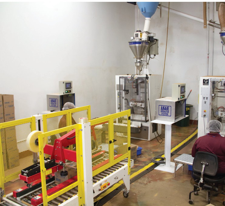
Iced tea concentrate for McDonald's rolls off two vf/f/s machines from General Packaging with operator station supplied by Automation Software & Engineering.
