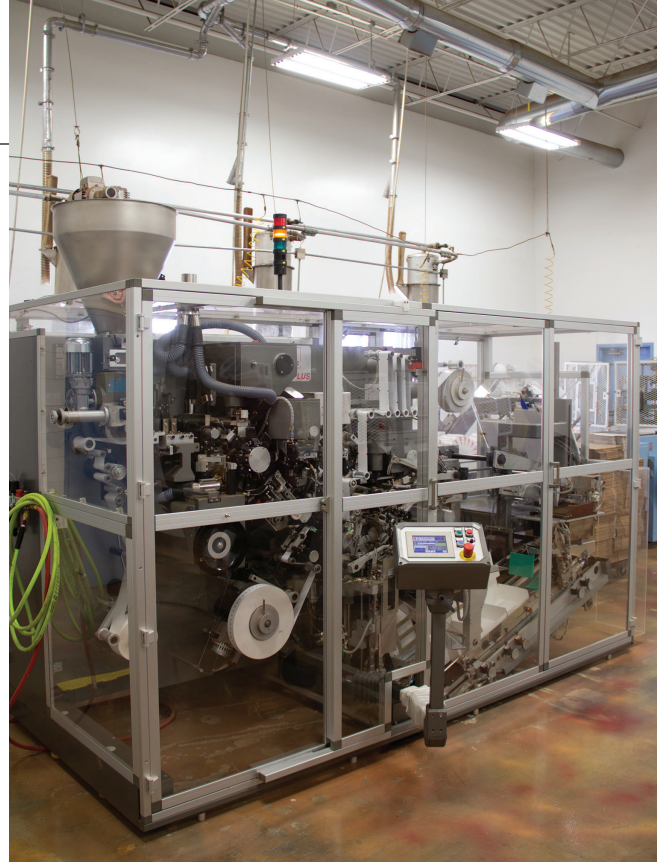
A new Model MD20 Plus from TeaMac increases throughput in a highly automated system with controls from Schneider Electric controls and a touchscreen interface from Pro-face.
